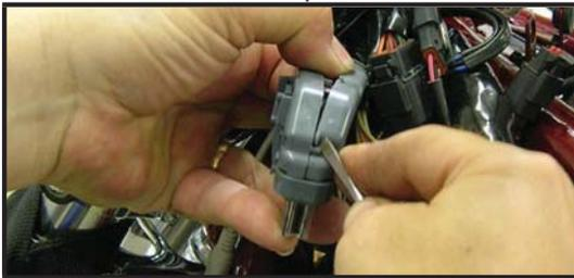
2. Depress the tabs on the connector retainer (clear plastic) and remove it from the connector.
