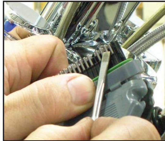
5. Re-install the connector retainer. Position the wires of the pigtail harness so that they exit the strain relief along the same path as the OEM wires. Close the halves of the strain relief around all the wires.
